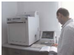
Digestor-extractor cu microscop MILESTONE ETHOS SEL CHIMIE-PROTMED
