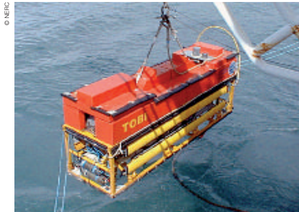
TOBI, a seafloor mapping system
