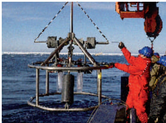
Multicorer for geochemical, sedimentological and micropaleontological sampling on board RV Polarstern
