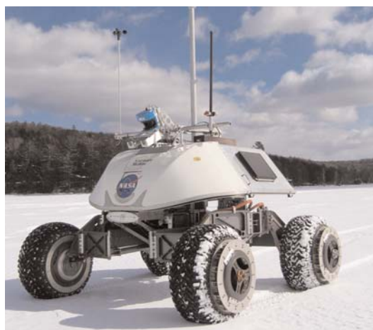
The experimental Life on Ice: Robotic Antarctic Explorer (LORAX) autonomous rover
