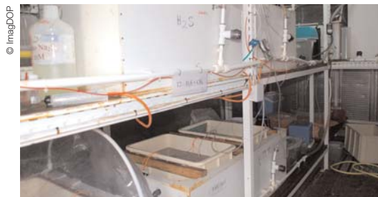
The LabHorta facility designed for the simulation of deep sea hydrothermal vents' conditions
